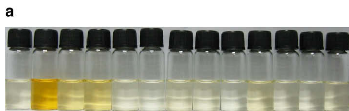
Figure 3. (a) The corresponding color changes and (b) absorption spectra when compound 1 (25 \mu\text{M} ) was treated with various anions (vials from the left: 1 only, \text{CN}^- , \text{F}^- , \text{AcO}^- , \text{H}_2\text{PO}_4^- , \text{HSO}_4^- , \text{Cl}^- , \text{Br}^- , \text{I}^- , \text{NO}_3^- , \text{ClO}_4^- , \text{SCN}^- , \text{N}_3^- ; \text{CN}^- , \text{F}^- , \text{AcO}^- , \text{H}_2\text{PO}_4^- , \text{HSO}_4^- : 1 equiv; \text{Cl}^- , \text{Br}^- , \text{I}^- , \text{NO}_3^- , \text{ClO}_4^- , \text{SCN}^- , \text{N}_3^- : 50 equiv) in \text{CH}_3\text{CN} - \text{H}_2\text{O} (97.5:2.5, v:v).
