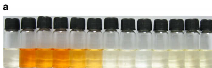
Figure 2. (a) The corresponding color changes and (b) absorption spectra when compound 1 (25 \mu\text{M} ) was treated with various anions (vials from the left: 1 only, \text{CN}^- , \text{F}^- , \text{AcO}^- , \text{H}_2\text{PO}_4^- , \text{HSO}_4^- , \text{Cl}^- , \text{Br}^- , \text{I}^- , \text{NO}_3^- , \text{ClO}_4^- , \text{SCN}^- , \text{N}_3^- ; \text{CN}^- , \text{F}^- , \text{AcO}^- , \text{H}_2\text{PO}_4^- , \text{HSO}_4^- , \text{NO}_3^- : 1 equiv; \text{Cl}^- , \text{Br}^- , \text{I}^- , \text{ClO}_4^- , \text{SCN}^- , \text{N}_3^- : 50 equiv) in \text{CH}_3\text{CN} .
